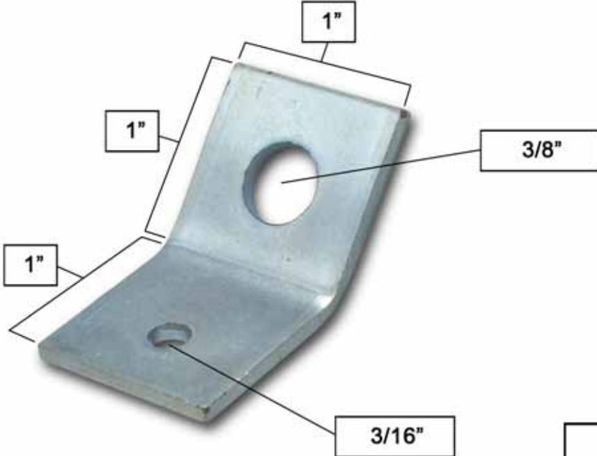
**Notes:** 45 degree 2 hole 12 gauge general purpose angle clip. Product weight 0.05 lbs. each, packaged 1,000 pcs per box. Complies with California DSA IR 25-2
